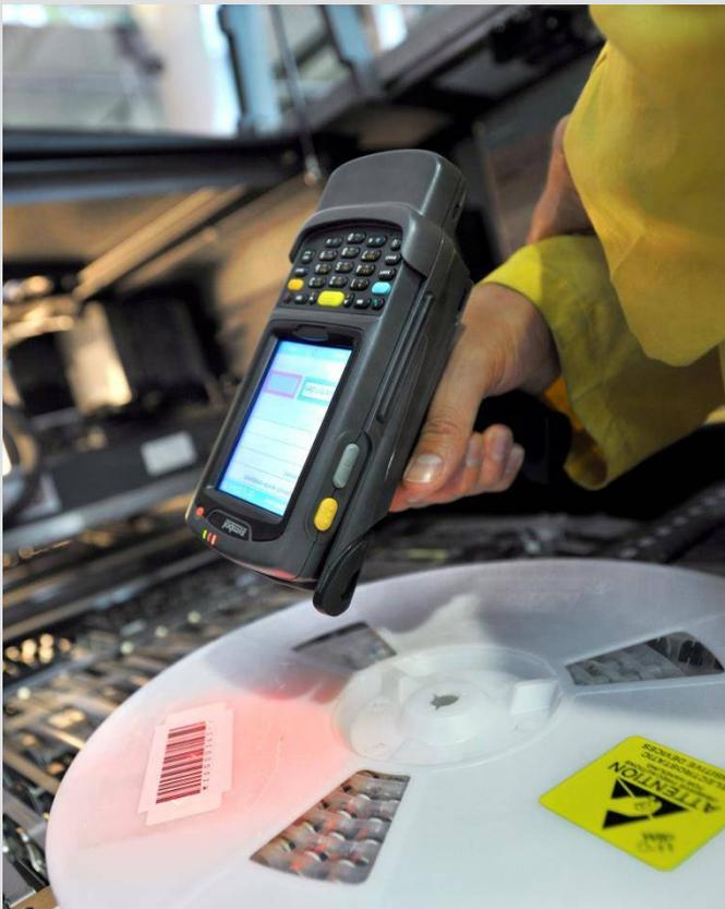
Your safety net against potential liability claims: ASM Traceability stores real-time information on assembled PCBs and placed components and allows you to analyze whether faulty input materials are responsible for defects in the finished products.
